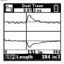
Dual Trace is used to compare two coaxial circuits at the same time (usually a faulted and a good circuit).
